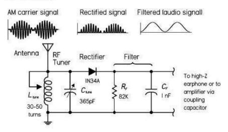
Output filter has time constant that is long compared to period of carrier, but short compared to period of audio signal.
