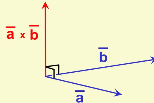
$$\bar{a} \times \bar{b} = (a_2b_3 - a_3b_2)\mathbf{i} - (a_1b_3 - a_3b_1)\mathbf{j} + (a_1b_2 - a_2b_1)\mathbf{k}$$
