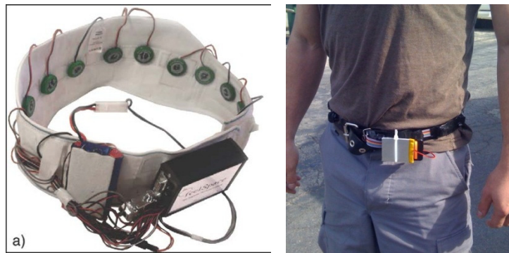
Haptic belt: Direction sense
