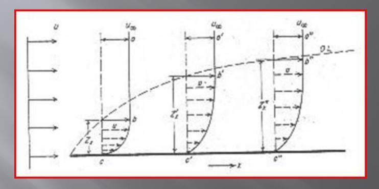
$$u \cdot \frac{\partial u}{\partial x} + v \cdot \frac{\partial u}{\partial y} = -\frac{1}{\rho} \cdot \frac{\partial P}{\partial x} + v \cdot \frac{\partial^2 u}{\partial y^2}$$
