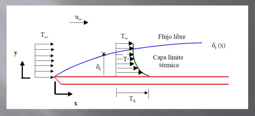
$$u \cdot \frac{\partial T}{\partial x} + v \cdot \frac{\partial T}{\partial y} = \alpha \frac{\partial^2 T}{\partial y} + \frac{v}{Cp} \cdot \left(\frac{\partial u}{\partial y}\right)^2$$
