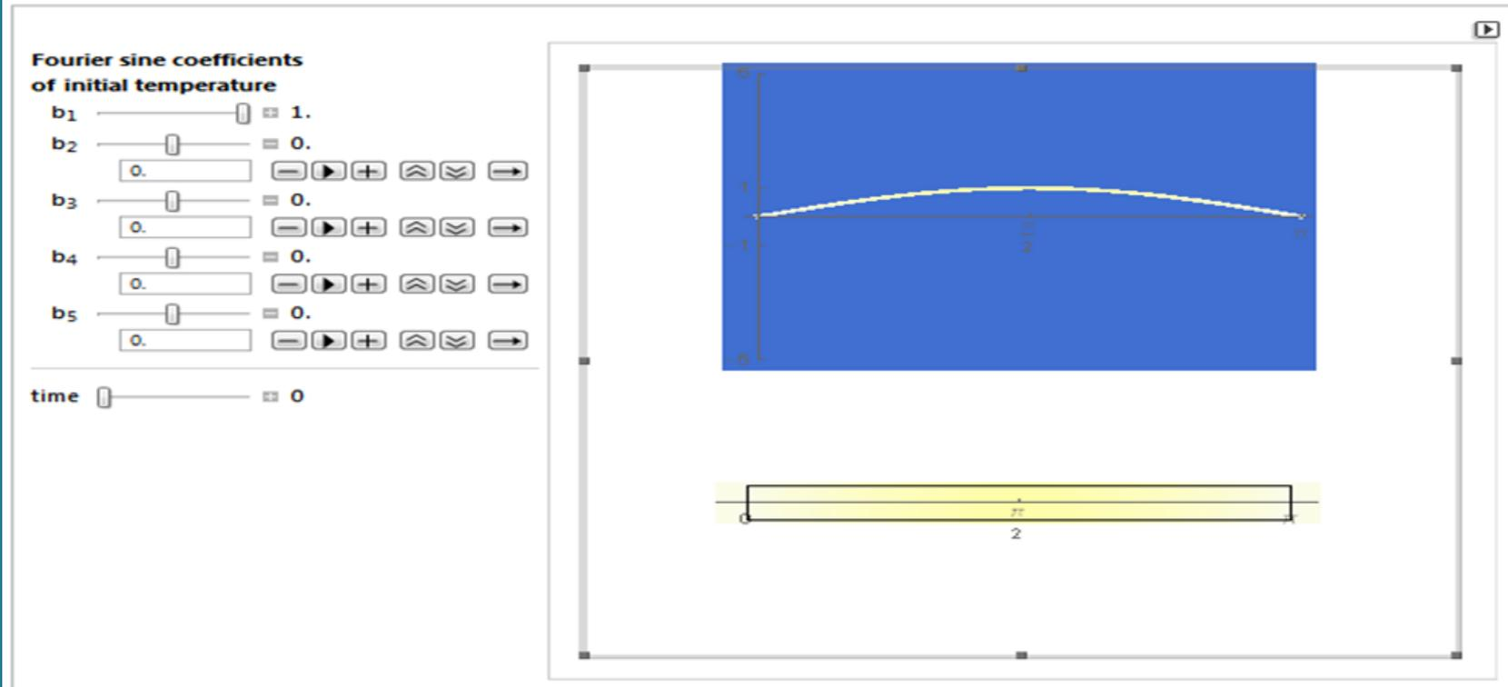
This Demonstration determines solutions to the mixed boundary-value problem for the one-dimensional heat equation. This pertains to the conduction of heat in a bar in which the ends are kept at fixed temperatures ( $0^\circ$  in this case), with a specified initial temperature distribution,  $u_0(x)$ .
